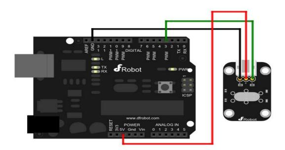
Interfacing And Connection With Moisture Sensor :
