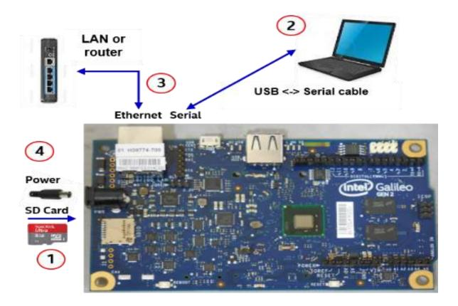
Figure : Intel Galileo Gen 2 Board
