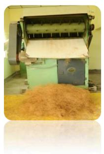
Input: Opened Fibers from Willowing M/c **Output:** Opened & Well Cleaned Fibers
