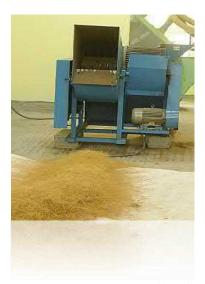
Input: Feed: Manual; Fibre flock; From side **Output:** Opened and moderately cleaned fiber
