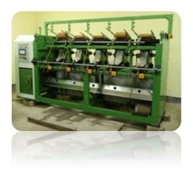
Input : Sliver from Slivering or Gilldraw Frame machine (As per Quality Req)
