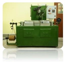
Input : Unsheared Single Yarn Output : Sheared Single yarn Production rate : 75 Kg/8 Hrs
