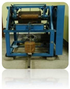
Input : Single or 2-ply yarn Bobbin Output : Large Yarn Spool of 5-10Kg.
