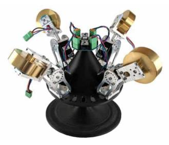
Control moment gyroscopes (CMGs) are a key technology for spacecraft attitude control. They are used to keep spacecraft stable and pointing in the desired direction. CMGs work by storing angular momentum. When a CMG is spun up, it acquires angular momentum. When the wheel is then commanded to stop spinning, it will exert a torque on the spacecraft in the opposite direction, causing the spacecraft to rotate.
