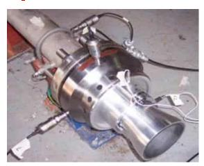
Cold gas thrusters are a type of rocket engine that uses the expansion of a pressurized gas to generate thrust. They are a simple and versatile propulsion system that is used in a variety of applications, including attitude control, maneuvering, and spacecraft propulsion.
