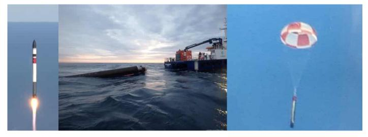
The first stage of Rocket Lab's Electron vehicle came down in a parachute-aided ocean splashdown on July 17. Rocket Lab launched seven satellites to orbit on July 17 and brought the booster back to Earth for a soft ocean splashdown. An Electron rocket carrying seven small satellites lifted off from Rocket Lab's New Zealand site 01:27 GMT on July 18, after being delayed by a few days due to bad weather.
