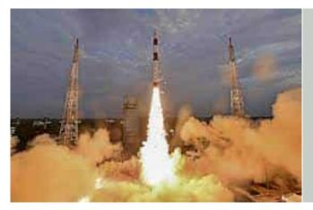
The launch of PSLV-C56 carrying DS-SAR satellite, along with 6 co-passengers from the first launch-pad of SDSC-SHAR, Sriharikota was accomplished successfully on July 30, 2023 at 06:30 hrs IST. PSLV-C56 is configured in its core-alone mode, similar to that of C55. It would launched DS-SAR, a 360 kg satellite into a Near-equatorial Orbit (NEO) at 5 degrees inclination and 535 km altitude.
