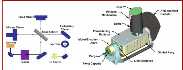
Infrared spectrometers are used in space to study the composition and temperature of objects in our solar system and beyond. They work by splitting light into its component wavelengths, or colors, and then measuring the strength of the light at each wavelength. This information can be used to identify the molecules that are present in an object, as well as to determine the temperature of the object.
