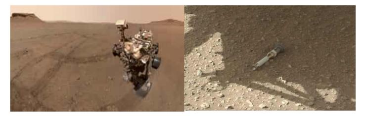
NASA's Perseverance Mars rover has finished building its backup sample depot on the Red Planet. The car-sized Perseverance rover just stashed the last of the 10 sample tubes that comprise the depot. Word of the successful drop came in on Jan. 29, about six weeks after the rover deployed the first of the samples.
