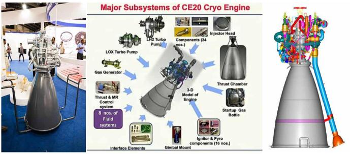
The Indian Space Research Organisation's (ISRO) CE-20 engine is an indigenous cryogenic engine that has propelled India's space program to new heights. This liquid-fueled rocket engine uses a mixture of liquid hydrogen and liquid oxygen as propellants, providing high thrust and excellent efficiency. With a thrust capability of 20 tonnes, the engine is designed to be used in the upper stages of the GSLV Mk-III rocket.
