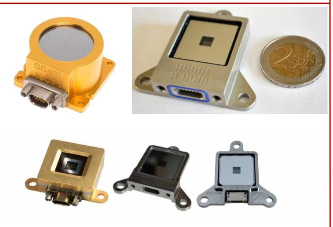
Sun sensors are small devices that play a critical role in space missions. They are used to measure the position of the sun relative to a spacecraft, which is important for determining the spacecraft's orientation and position in space.
