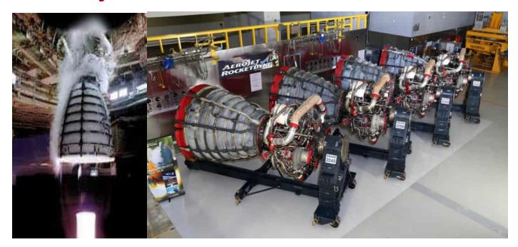
The RS-25 engine, also known as the Space Shuttle Main Engine, is one of the most powerful and efficient rocket engines ever developed. Developed by NASA and Pratt & Whitney Rocketdyne, the engine was originally designed to power the Space Shuttle. Today, it continues to play a critical role in space exploration, powering NASA's Space Launch System (SLS) rocket.
