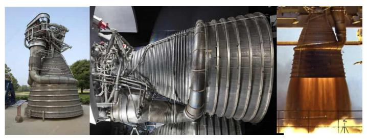
The F-1 engine was a marvel of engineering and a critical component of the Saturn V rocket that took astronauts to the moon. Developed by Rocketdyne in the 1960s, the F-1 engine was the most powerful single-chamber liquid-fueled rocket engine ever built, producing a staggering 1.5 million pounds of thrust at liftoff.
