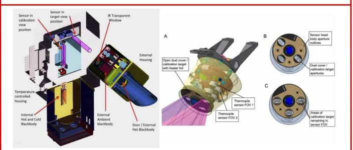
Radiometers have played a crucial role in our understanding of the Earth's climate and the composition of the universe. These instruments are used to measure the intensity and spectrum of electromagnetic radiation emitted or absorbed by objects in space. Radiometers used in space are equipped with specialized detectors that can measure radiation across a wide range of wavelengths, from visible light to microwave and radio frequencies.
